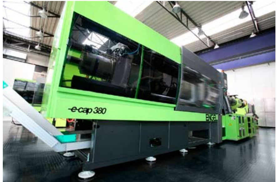
With extremely short cycle times of less than two seconds, the new e-cap ensures very high precision and repeatability. (Pictures: ENGEL)
