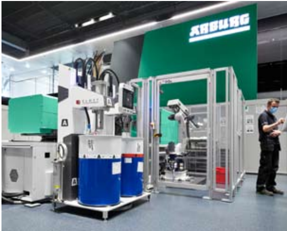
Two Allrounders manufacture the LSR and PP components. The individual parts are manually assembled to form the high-quality, high-tech mask, which Arburg developed itself and realised with partners. The soft LSR component is produced by an electric Allrounder 570 A.
