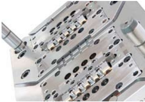
A 16-cavity mold with two TFS-Linear with 4+4 injection points (© Thermoplay)
